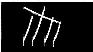
Fig. 4-11. Waveform with alternate symmetry.
