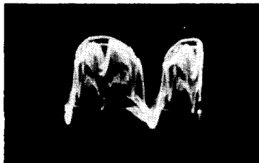
Fig. 4-6. Noise-gate signal applied to point F.
