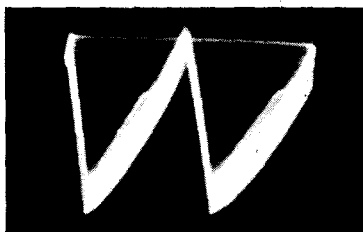
Fig. 5-6. Distorted waveform appears at (B) when C1 is open.
