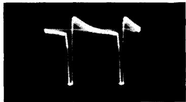
Fig. 5-19. Mixed pulse and sawtooth waveform.
