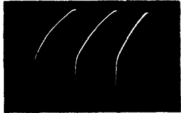
Fig. 7-16. Input waveform to the vertical-blanking network.
