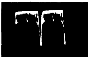
Fig. 4-5. Unsatisfactory sync separation.
