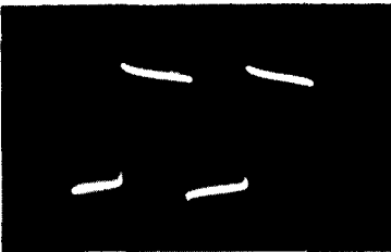
Fig. 11-11. Tilt in the top of a square wave is caused by low-frequency attenuation and phase shift.
