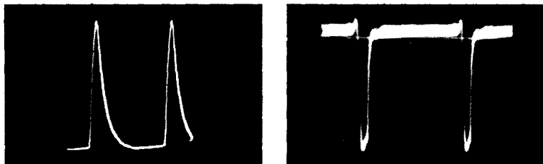
Fig. 4-15. Sync-separator outputs from two different receivers.
