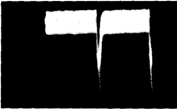
Fig. 4-16. Excessive residual video in the stripped-sync waveform.
